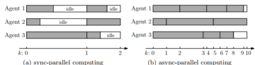
Figure 2: Sync-parallel computing (left) versus async-parallel computing (right). On the left, all the agents must wait at idle (white boxes) until the slowest agent has finished.
